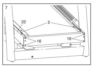
8. Attach the Front Cover (17) to the Frame (22) with the two Cover Screws (2) and the four Front Cover Screws (16).
