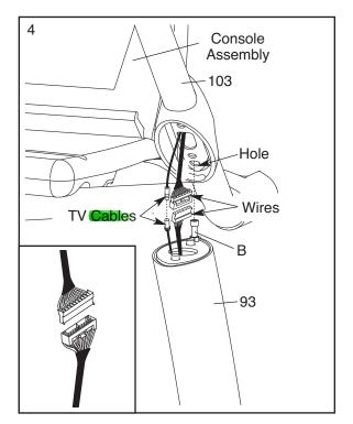
5. With the help of a second person, pivot the console assembly to the position shown. **Be careful to avoid pinching your hands or the wires.**
