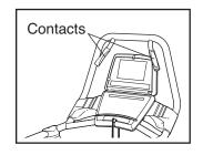
palms must be resting on the upper contacts, and your fingers must be touching the lower contacts. **Avoid moving your hands.** When your pulse is detected, the PULSE indicator above the main display will begin to flash, and then your heart rate will be shown. For the most accurate heart rate reading, hold the contacts for at least 15 seconds without moving your hands.
