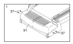
Using a hand-held vacuum, clean the area under the Motor Hood (not shown). Be careful to avoid touching any components. Check the Motor Belt (82) for wear and cracks. If the motor belt needs to be replaced, please see the back cover of this manual.
