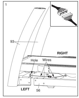
Slide the Uprights (93) onto the Base Frame (56), and align the holes in the Uprights with the holes in the Base Frame. Be careful to avoid pinching the wires. Finger tighten two Side Base Bolts (95) through the bracket near the right Upright and into the Base Frame; do not tighten the Side Base Bolts yet.
